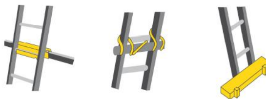
Some effective ways of securing the top and bottom rungs of straight ladders
